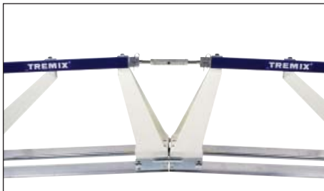
The quick couplings can be adjusted up to a +/- 5% angle to allow slopes in the slab. As an option the couplings can be replaced by a special connection for further angling up to +/-30%.
